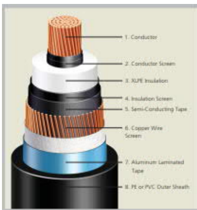
Figure 4.4: Indicative Land Cable Design
