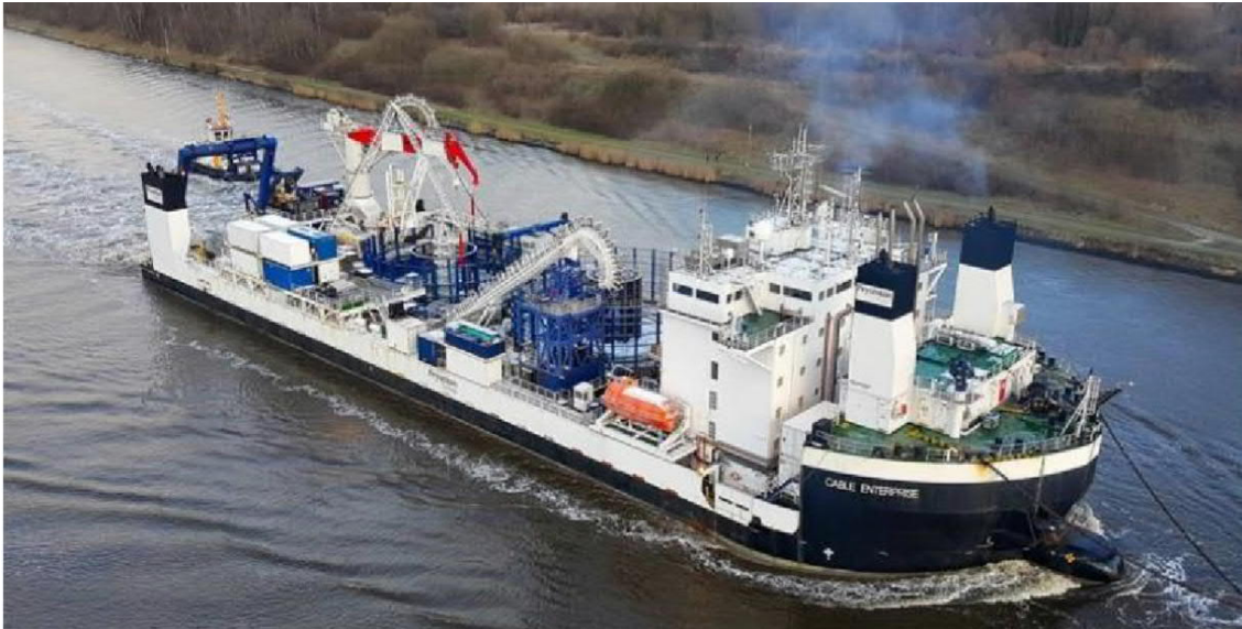
Figure 4.20: Example of a primary Cable Laying Barge [approximate size 125m (l) x 32m (b)]
