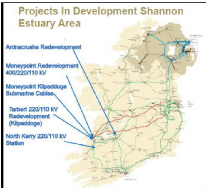
Figure 2.3: Projects in Development Shannon Estuary Area (Reproduced Figure 5.20 of the SEA Environmental Report)
