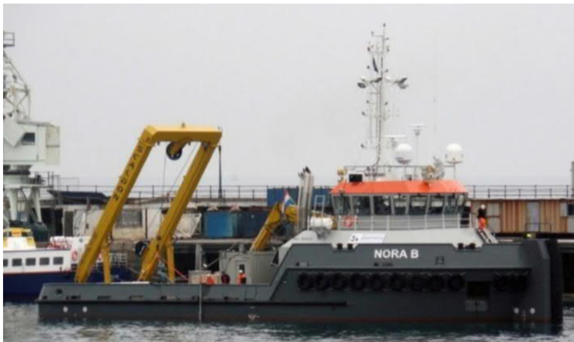
Figure 4.22: Example of a Pre-Lay Grapnel launch vessel
