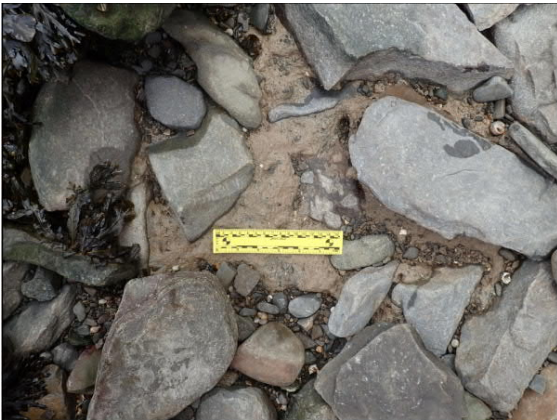
Figure 11.10: Detail shot showing exposed Clay (Glacial Till) located below the foreshore deposits at the proposed northern landfall (150mm scale)
