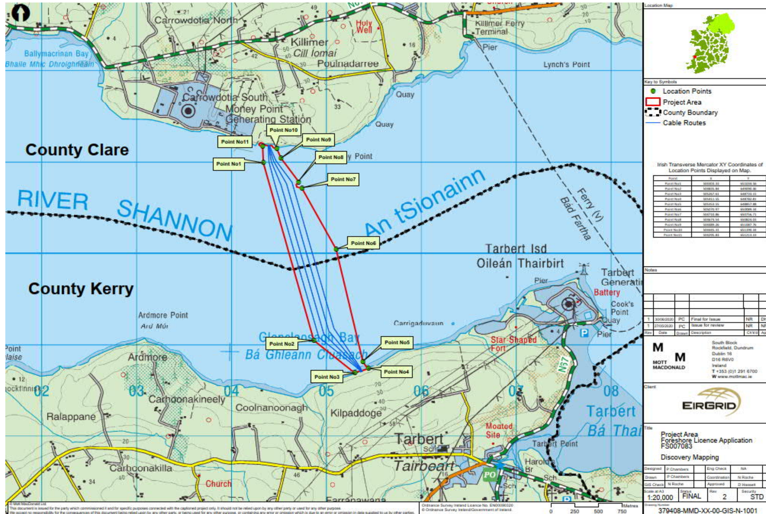
Figure 4.8: Proposed Alignment of the submarine cable route
