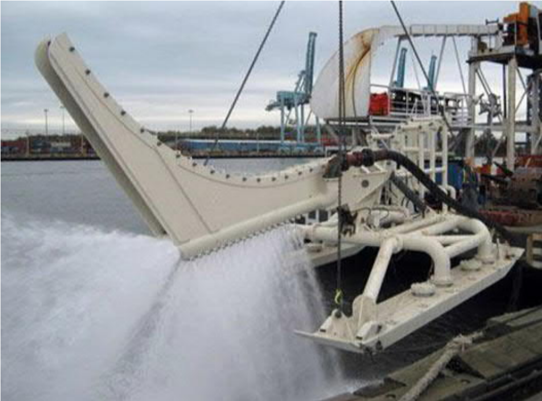
Figure 4.24: An example of a jetting tool
