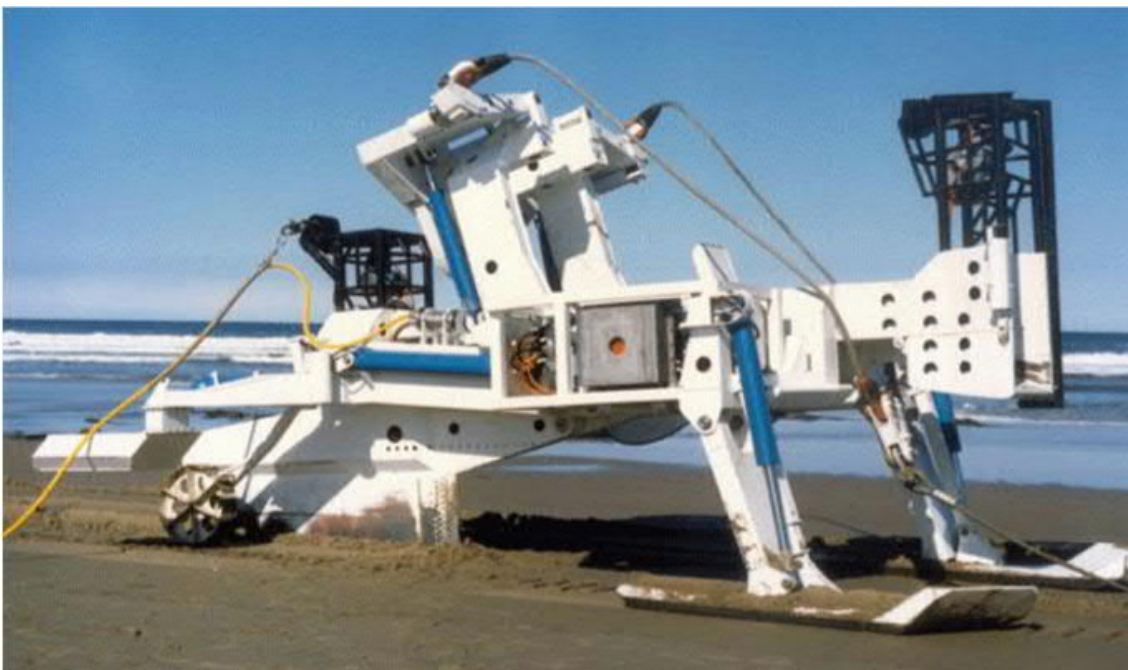
Figure 4.21: Example of a cable burial tool
