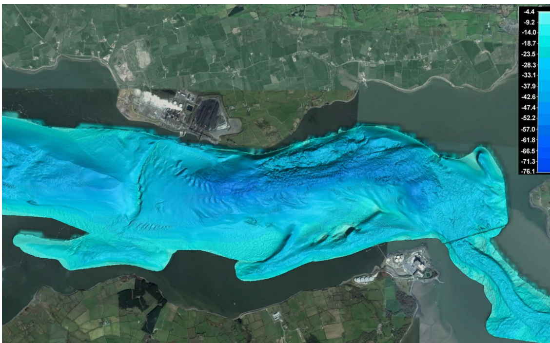
Figure 7.14: Multibeam data of the cable laying area
